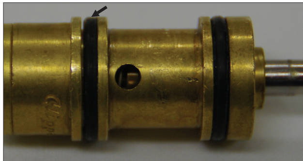
Fig. 1. An enlarged mechanical part of oxygen flush valve. We found the rubber of O-ring was worn out (arrow).
