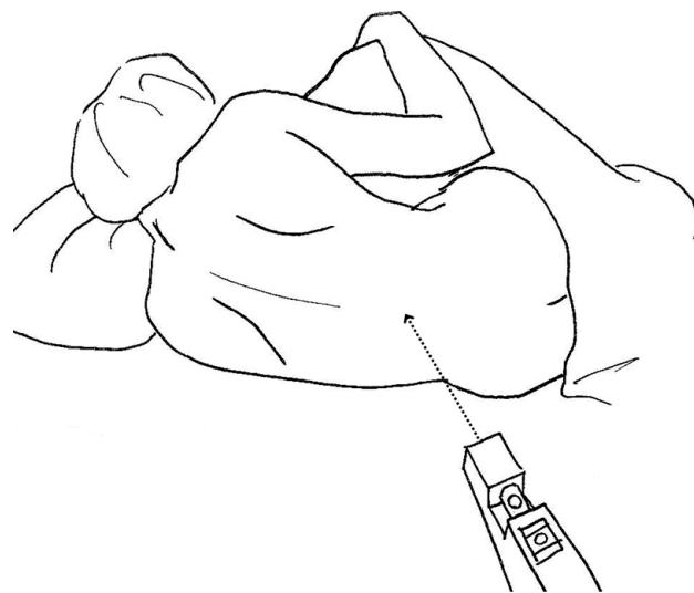
Fig. 1. Illustration of a laser leveling device. The zero level of a pressure transducer is set at the insertion point of Tuohy needle.
