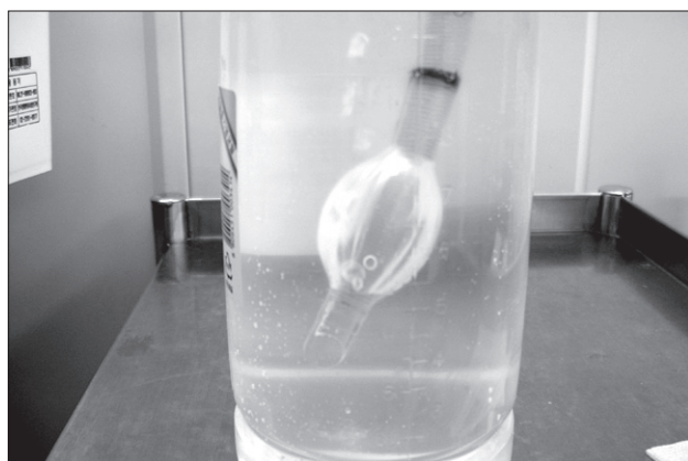
Fig. 3. The air bubbles coming out of the lower parts of endotracheal tube cuff are seen. There were two points of 1–2 mm sized lacerations on lower part of the cuff.
